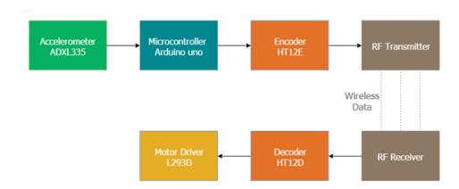
Here the accelerometer reads the X Y Z coordinates when we make gestures by hand and send the X Y Z coordinates to the Arduino (here we don't need the Z axis we need only two coordinated X and Y So neglect the Z coordinate). The Arduino checks the values of coordinates and sends a 4 bit code to the Encoder IC. The Encoder passes the data to RF transmitter and the transmitted data is received by the RF receiver. The receiver sends the 4 bit code to the Decoder
