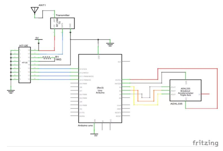
It consists of Arduino Uno , ADXL335 Accelerometer , Encoder IC and a Transmitter module . The signals from the accelerometer is fed to the analog pins of arduino. Arduino has an inbuilt analog to digital coverter (ADC). The encoder it into machine readable form. And finally the transmitter will transfer the signal to the robot.
