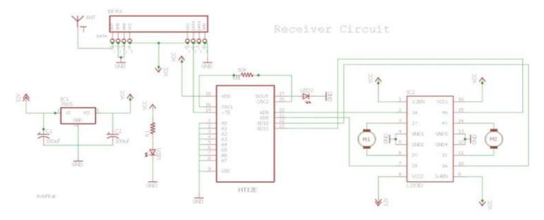
The receiver circuit consists of 2 IC (HT12D decoder, L293D motor driver), RF receiver module.
